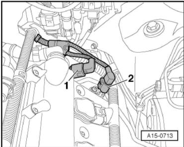
Connect multimeter for voltage measurement as follows:
