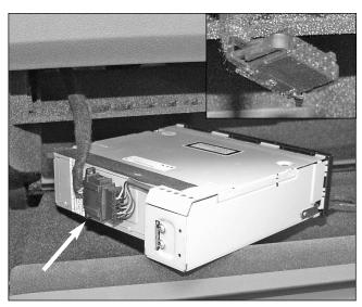
Step#4: Vehicles with CD Changer: Disconnect CD harness connector from the rear of the CD Changer. Set the CD Changer aside.
