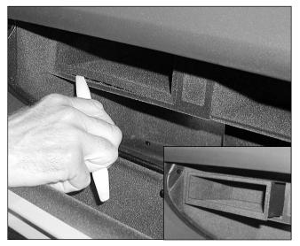
Step#1: Vehicles with CD Changer Prep: Using plastic trim tool, remove glove compartment insert.
