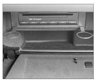
Step#3: Vehicles with CD Changer: Using 3B7 051 530 removing tool, remove the CD Changer.
