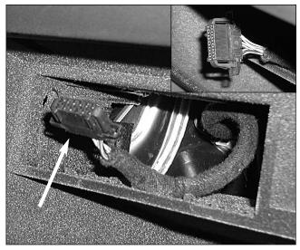
Step#2: Vehicles with CD Changer Prep: Disconnect CD harness connector from the rear of the glove compartment insert. Place glove compartment insert aside.
