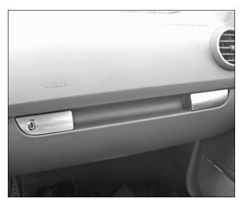
Step#13 Return the glove compartment to closed position, remove any fingerprints or debris. Unless otherwise instructed, provide the insert and i Pod® Interface adapter trays and shims to owner.
