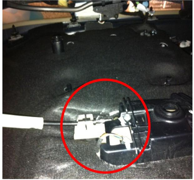
3. With the panel off you need to remove the liner, which sits with some special washers that just unscrew
