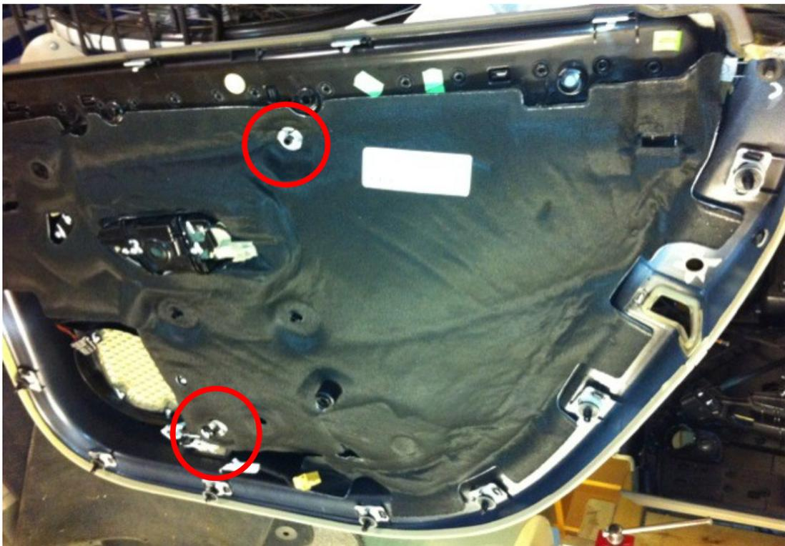
When liner's gone you can access the screws to handels, speaker grilles etc etc. I'm looking to replace the handles so then there are 11 T20 screws to remove
